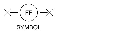
FILTER FABRIC FENCE NTS
